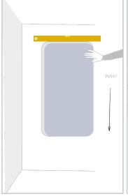
**3. Gently** place the absorber. Let it touch the wall only with the upper edge at first. Confirm that the absorber is **straight using spirit level**. Push to attach.
