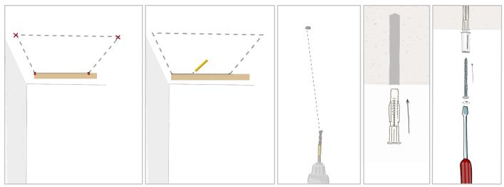
1. Choose the best place for your absorber. Mark the spots for drilling. To be sure you can measure the distances between the dowels inserted in the absorber and see if your marks has the same distances.
