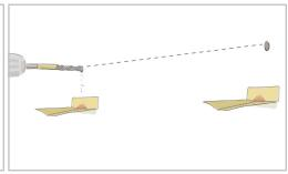
5. To eliminate mess from the crumbling wall while drilling, place **sticky notes** sheets under the marked spots.
