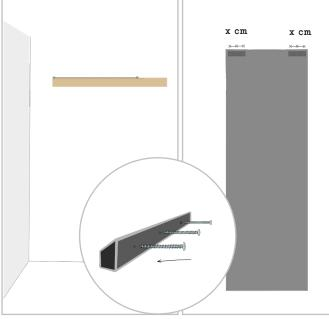
**3. Mark the spots** where you'll need to drill holes for the plugs and screws in the wall.
