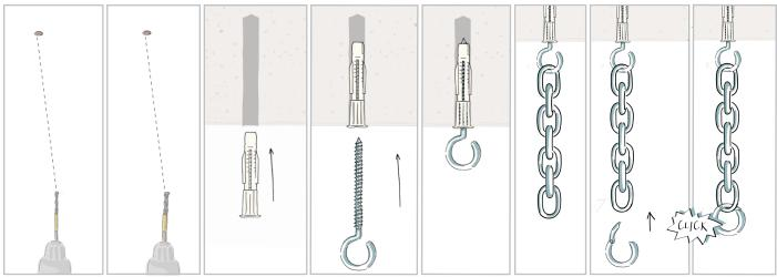
**6.** Drill holes on the marked spots. Use the **smaller drill first** to avoid bigger damage on plaster and masonry. Repeat drilling with the **6 mm drill size** = the **same** size **as your plugs.**
